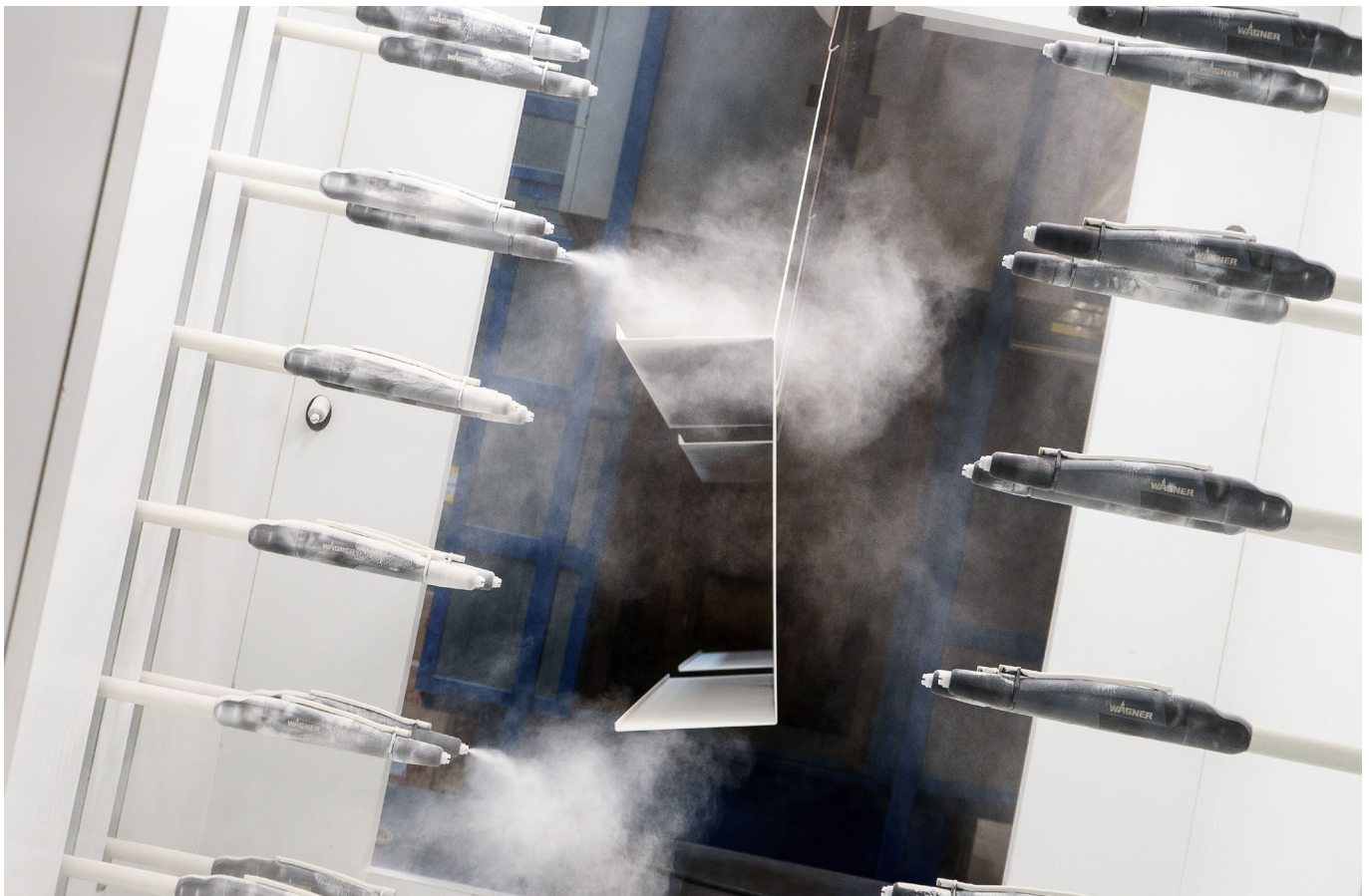
Powder coating: After a series of rinse zones the workpiece is finalized with an electrical charge, that is highly dependent on the pureness of the water. The correct water quality is essential for the pretreatment process, regardless if it is for e-coat, powder coating or liquid paint.
